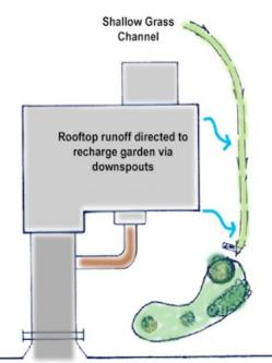
• Tree and Shrub Pits Stormwater management technique that intercepts runoff and provides shallow ponding in a dished mulched area around the tree or shrub.
