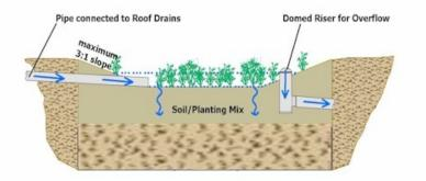
A Rain Garden (also called Bioretention) is an excavated shallow surface depression planted with specially selected native vegetation to treat and capture runoff.
